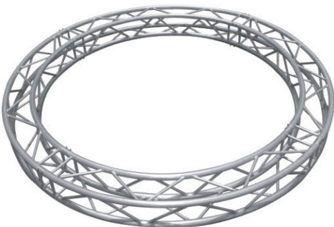
SCT-290 Square Circle Truss 50mm/3mm Diameter: 1M - 15M
